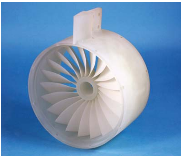
MIT Engineers created CAD models of “Vaned Disks” which were manufactured by Solid Concepts utilizing SLA rapid prototyping technology.
