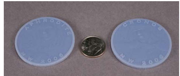
The PolyJet process results in excellent up facing and down facing surfaces.
