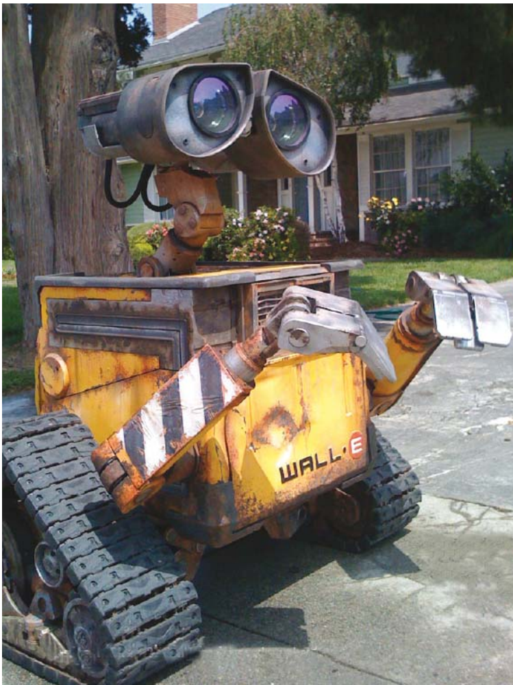
Physical WALL-E, a real robot built with SLA for tours, guest appearances, and trade shows.
