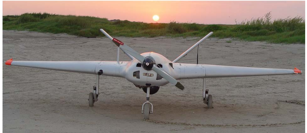
The DRS Sentry HP has a wingspan of 12.8 ft. and can accommodate various internal payloads of up to 75 lbs. for military and civilian applications. The aircraft is controlled through a sophisticated digital flight control system and integral mission computer.
