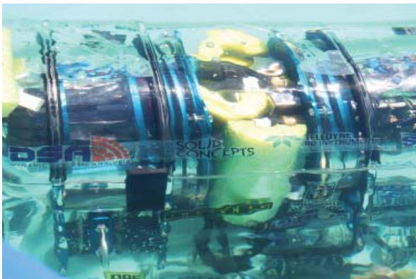
AUVic's UUV needed to be water tight and strong enough to handle the pressures produced under water.
