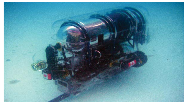
AUVic's ultra compact UUV vehicle hybrid can function as an AUV, intelligent ROV or a combination of both.
