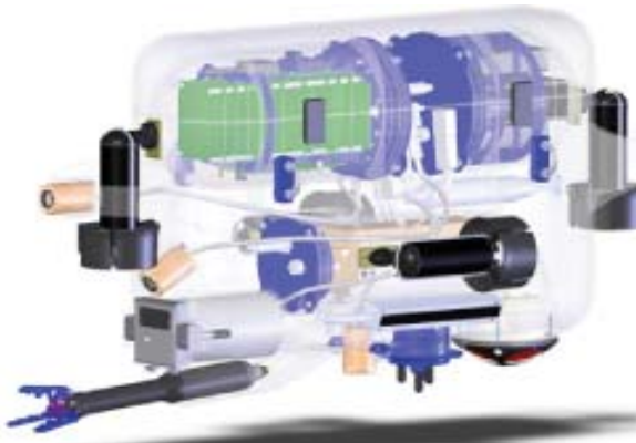
CAD image showing the mechanical features of the AUVic's UUV design and housing.
